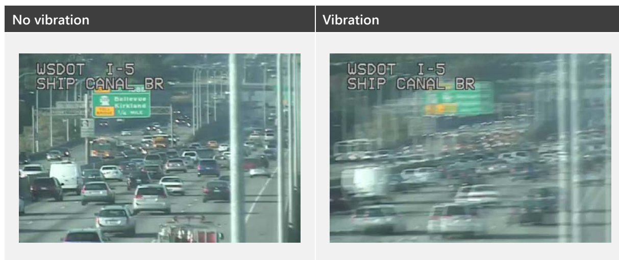
Figure 2-7: Vibration effects on CCTV image
