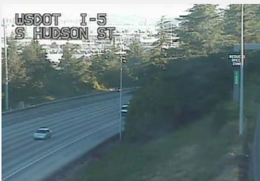
Figure 2-4: Poor coverage due to vegetation growth
