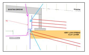
micropiles are installed, nailing and excavation would continue. There would probably be two rows of long nails that would also help restrain the tops of the micropiles. As shown in the image to the right.
